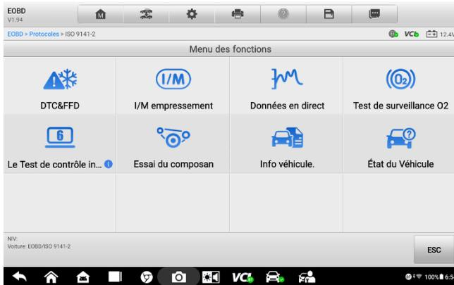
**Figure 4-15 Menu Diagnostics OBDII**
